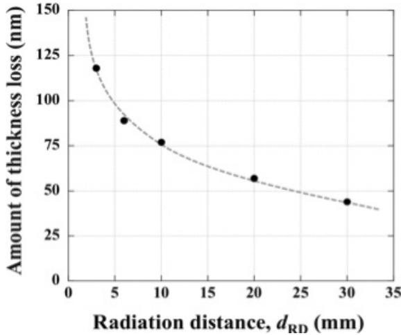
Fig. 3. Effect of radiation distance by VUV-exposure.
