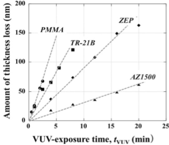
Fig. 1. Thickness loss of various resins by VUV-exposure.
