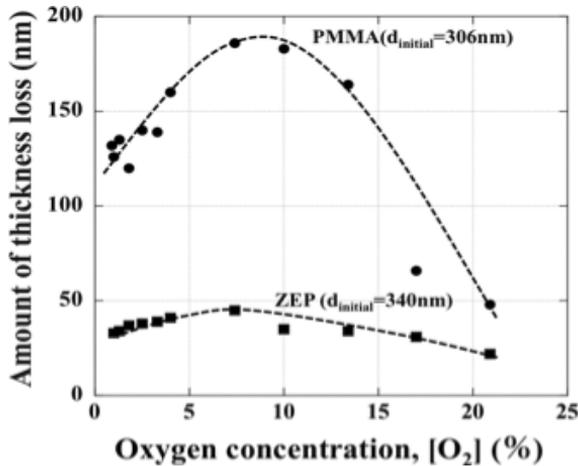
Fig. 4. Effect of ambient oxygen concentration by VUV-exposure.
