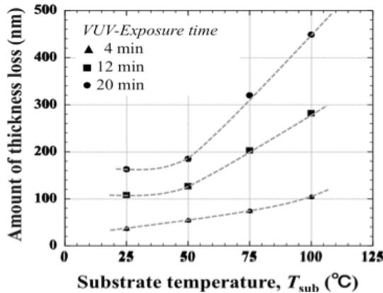
Fig. 2. Effect of Substrate temperature by VUV exposure.
